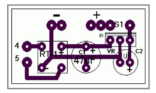
The circuit shown below is a combination of an adjustable resistance with a Zener diode which will enable adjustment of a regulated voltage, note that you will not be able to lower the voltage below the zener's voltage value. This type of regulation will allow you to use higher current output than a single regulator IC as described previously which is limited to 1.5A. For still higher current output an additional identical transistor can be connected in parallel.
