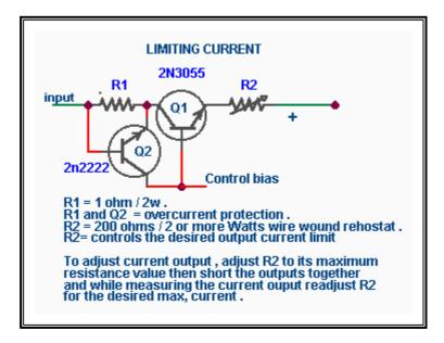
There are other ways to protect your power supply? The next two circuits are electronic fuses or rather current fold back circuits which when connected in series with your power supply will shut down your supply system when any
